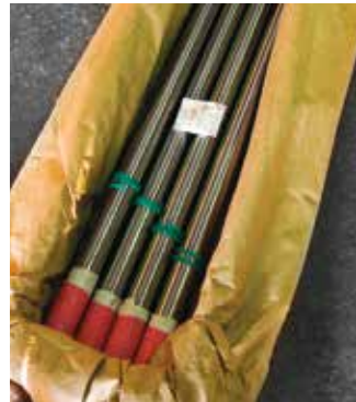
Bars wrapped in moisture absorbing paper
